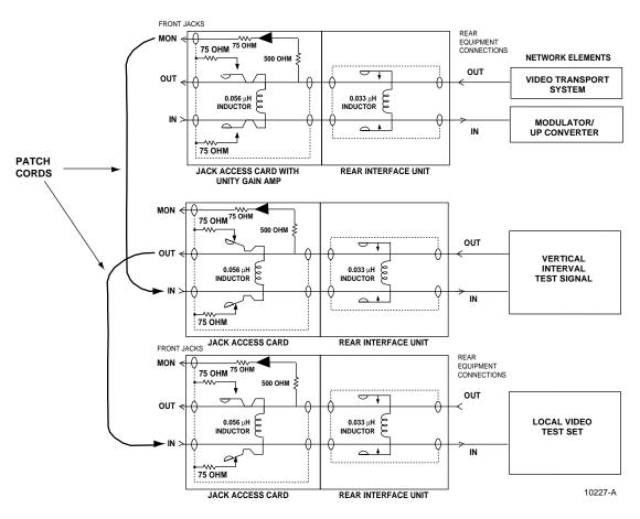
Figure 32. Non-Intrusive Insertion of Video Test Signal
